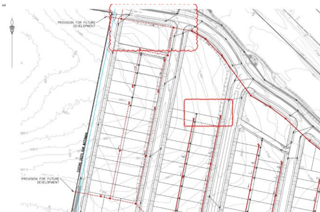
Figure 8 Sewer master plan - Sheet 3 Source: Colliers
