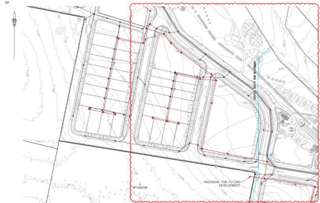
Figure 7 Sewer master plan - Sheet 2 Source: Colliers
